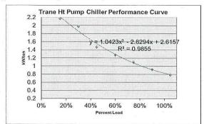
Figure 1: Existing Heat Pump Chiller Performance Curve
